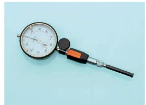
OSG measuring gauge for internal threads
