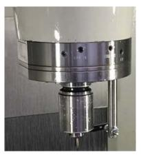
Whenever possible, it is always recommended to use the orientation lever, which is supplied with the machine, as it solves a number of problems during machining.
