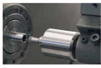
When machining on a CNC lathe, in most cases it is not possible to use the drive lever (unless you are using a 'motorised' one) as there are usually other machining operations before or after using the Poliangolar unit. In this case, broaching can still be carried out by starting machining in another way:
